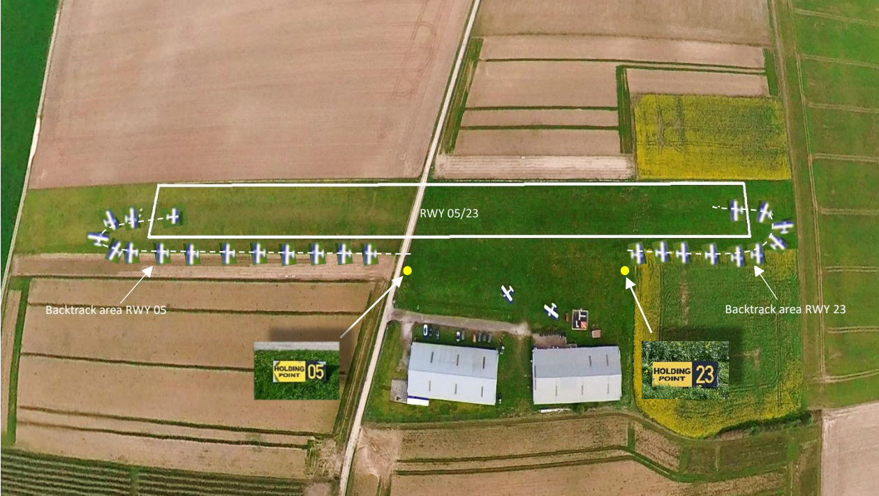
Holding points and backtrack area
